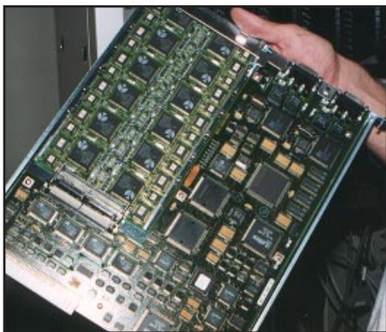
Twelve new modems for TIP (upper left of board)
