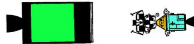
5 CSM and LM separate from last stage of Saturn rocket
